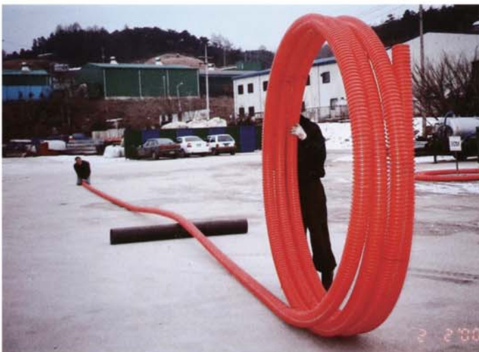
▲ COD by-passes hurdles owing to its flexibility
